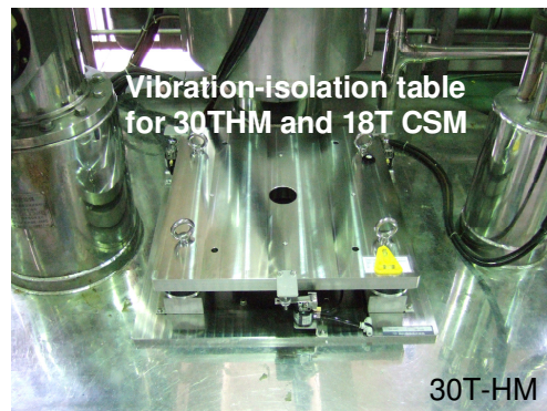
Fig. 1 Non-magnetic vibration-isolation table for 30T-HM and 18T-CSM.
