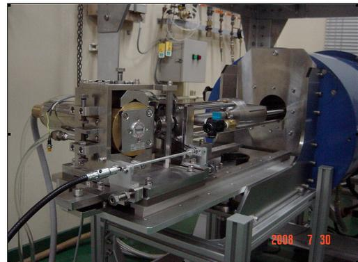
Fig.2 Photo of the high-field X-ray powder diffraction camera that is combined with a 10T-100mm bore cryocooled superconducting magnet.
