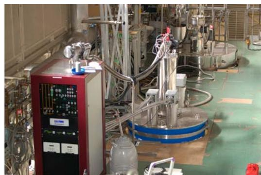
Fig. 1. Sliding seal type dilution refrigerator for the cryogen-free hybrid magnet. The gas handling system can be controlled from an operation room.
