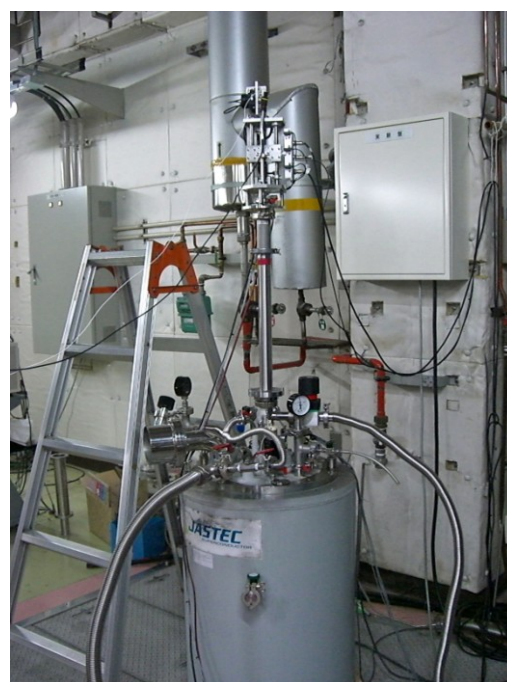
Figure 2. 18 Tesla extraction type magnetometer in the High Field Laboratory for Superconducting Materials, Institute for Materials Research, Tohoku University, Japan.
