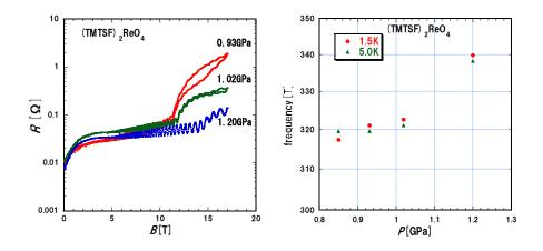
A single series of rapid oscillations (RO) in the metallic and the field-induced spin-density-wave (FISDW) state with two anion ordering (AO2, AO3) in (TMTSF)<sub>2</sub>ReO<sub>4</sub> for various pressures was investigated through transport measurements under magnetic fields. With increasing pressure, (i) the oscillation frequency of RO slowly increases below 1.1 GPa, (ii) the frequency rapidly increases above 1.1 GPa. This behavior is related to the disappearance of AO2 above 1.1 GPa.
