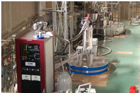
Fig. 1 . Dilution refrigerator for the cryogen-free hybrid magnet.
